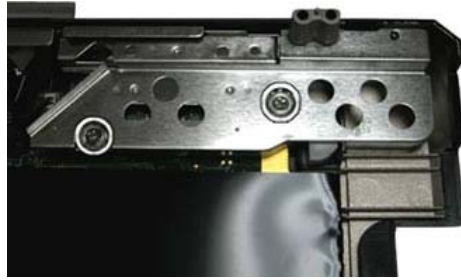
Fig. 30 Removing the Versa Bay shield
